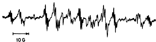
Figure 1. 9.4 GHz E.s.r. spectrum from a mixture of cis - and trans -4- t -butylcyclohexylmethyl bromides in propane at 115 K. Some lines from the isopropyl radical, derived from the solvent, can also be observed
